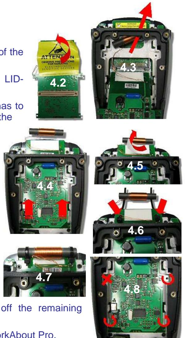
Use the 4 screws to secure the LID-WAP into the WorkAbout Pro.
