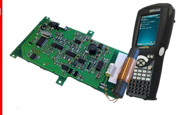
The LID-WAP version 2 decoder is especially designed for the PSION Workabout Pro. It is easy to install on the 100 pin High speed expansion interface.
