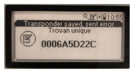
In this case, the ID number is stored with date and time. The reader has not send the ID number via BLE to an external device.
