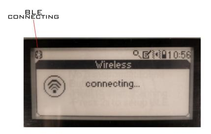
When the reader is connected via BLE to the external device it is visible in the display via the icon in the left upper corner[1], after a tag is read the reader will try to connect to the paired device [2].
